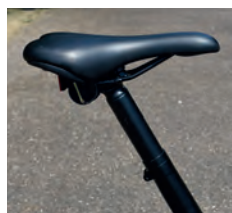
Top: Supernova LED lights are wired in to the main battery Bottom: As well as a telescopic seatpost, the seat angle is slacker so the reach extends more for taller riders
