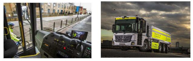
"Direct vision" lorry cabs, in which drivers can see what is around them as easily as a bus driver can, with the driver seated down low and surrounded by as much window as possible.
