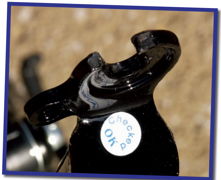
One fork end was a bit crushed and needed fixing
