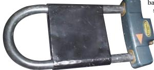
After reading the security article in the Feb-Mar issue of Cycle, I asked a local smithy to make for me a lightweight steel box to fill the inside of my D-lock to prevent access with a 'stubby' bottle jack. It is made from thin-gauge steel, MIG-welded, and slips on between bike and locking post as shown.
