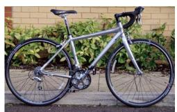
The Pilot 2.0 says it's designed with comfort in mind, with an extended head tube to allow higher handlebars without increasing standover height. I felt it was a great bike both for fast commuting (a higher eye-level is good in traffic) and audax or sportive rides, where comfort over long distances is essential.
