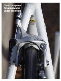
puts cable adjusters on the levers instead of the frame. They're handy there but limit this bike's upgradeability to any system which routes gear cables under the tape.
