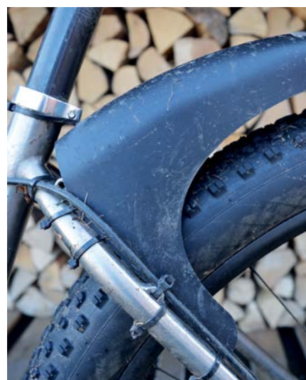
Above: Unlike seatpost brackets, which can rotate or snap off, cable-ties stay put, making the Mudhugger stable and secure
