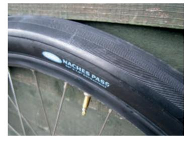
FFERED IN STANDARD and Extralight formats, weighing 350g and 300g respectively, the Naches Pass is one of a wide range of tyres from a US brand that has recently led the trend for exceptionally light, wider-section road – or, as Compass would put it, 'allroad' – tyres. The range includes tyres to fit 26-inch, 650B and 700C rims (ISO 559, 584 and 622).
